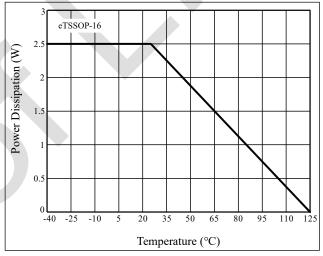
Figure 16 Dissipation Curve
