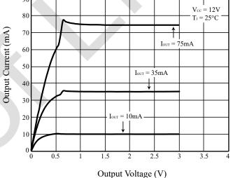
Figure 11 Output Current vs. Output Voltage
