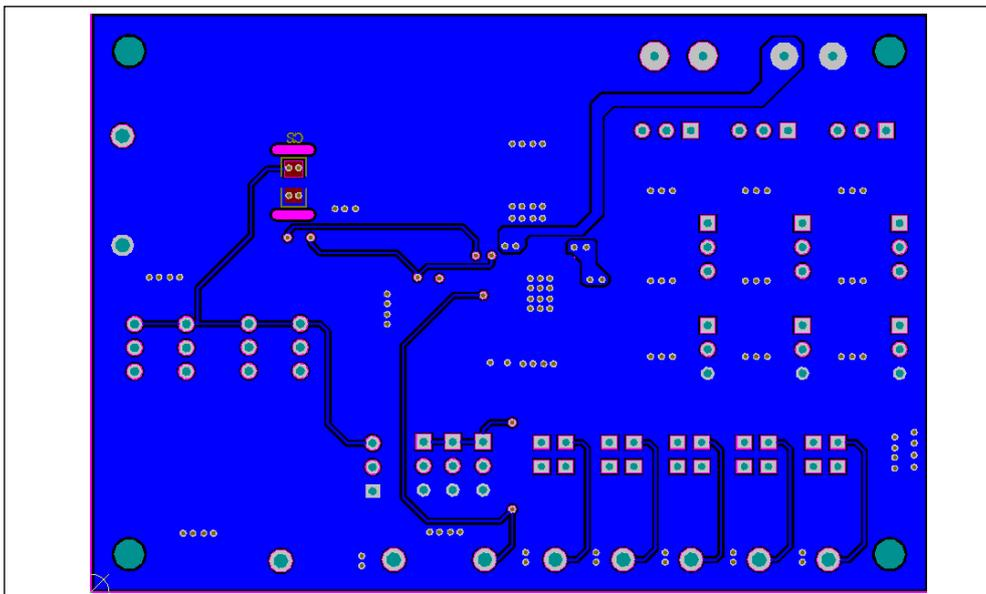
Figure 9: Board PCB Layout - Bottom Layer
