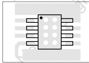
Figure 35 Board Via Layout For Thermal Dissipation
