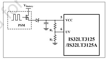
Figure 32 UV Pin Operation
