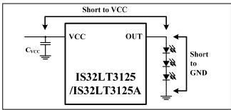
Figure 33 OUT Pin Shorted Operation
