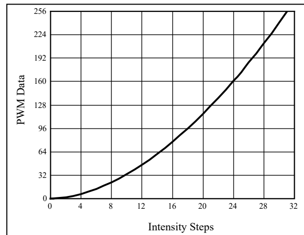
Figure 6 Gamma Correction (32 Steps)
