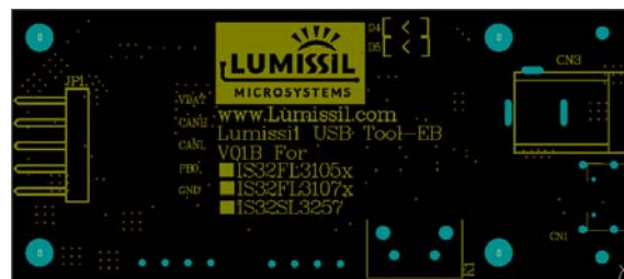
Figure 14 Board Component Placement Guide - Bottom Layer
