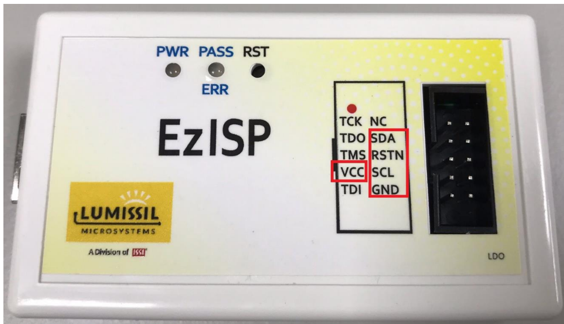
Figure 9-2: Pin configuration on EzISP board
