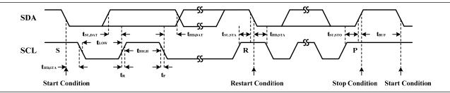
Figure 6 I2C Interface Timing
