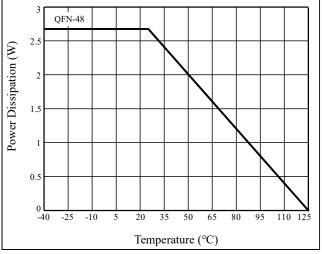
Figure 16 Dissipation Curve
