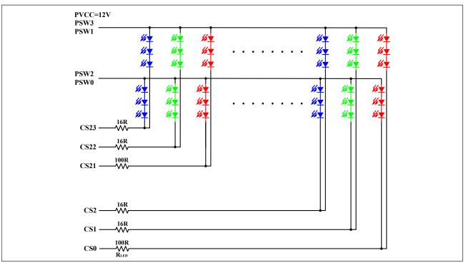
Figure 5 LED Circuit: 24×2
