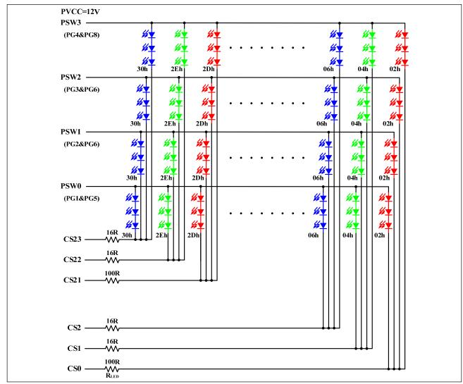
Figure 3 LED Circuit: 24×4
