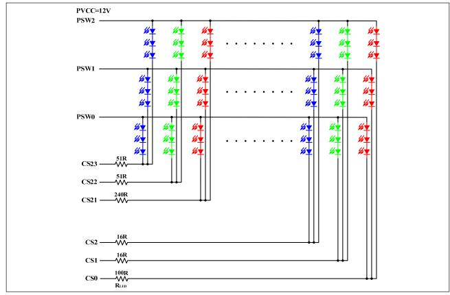
Figure 4 LED Circuit: 24×3
