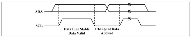
Figure 7 I2C Bit Transfer
