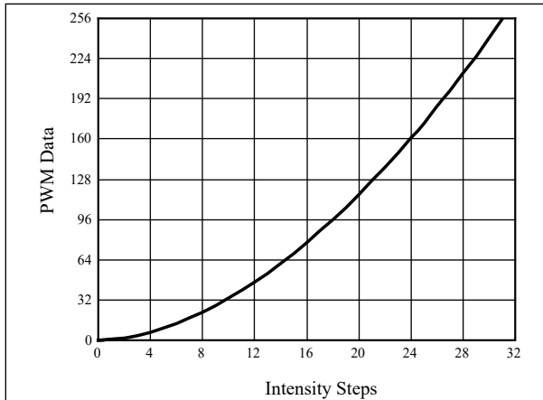
Figure 15 Gamma Correction (32 Steps)
