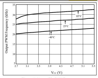
Figure 18  $V_{CC}$  vs. CSx PWM Frequency
