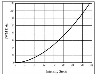
Figure 13 Gamma Correction (32 Steps)
