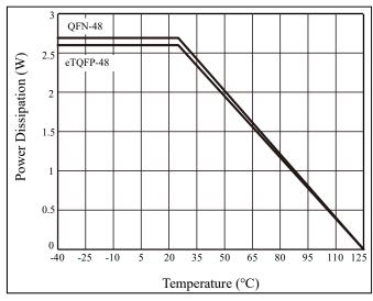
Figure 17 Dissipation Curve
