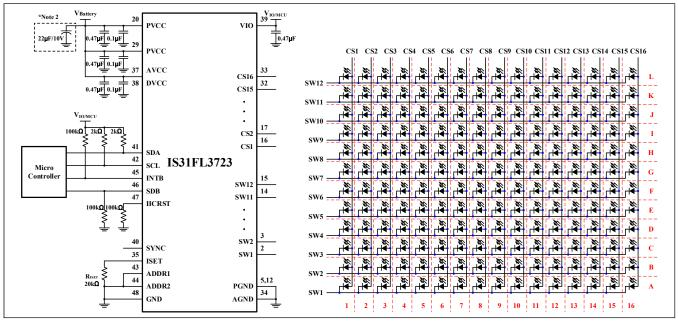
Figure 1 Typical Application Circuit (12×16)
