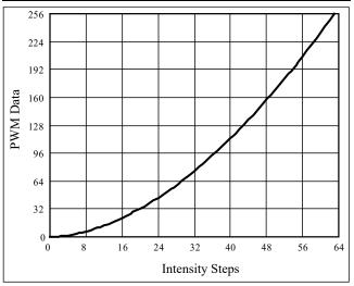
Figure 14 Gamma Correction (64 Steps)
