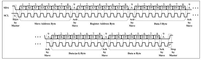
Figure 7 Writing to IS31FL3723 (Automatic Address Increment)
