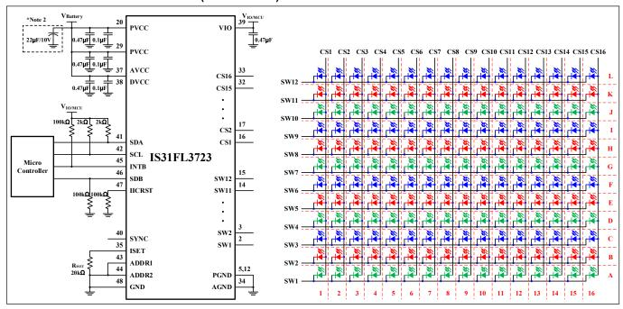
Figure 2 Typical Application Circuit (RGB)
