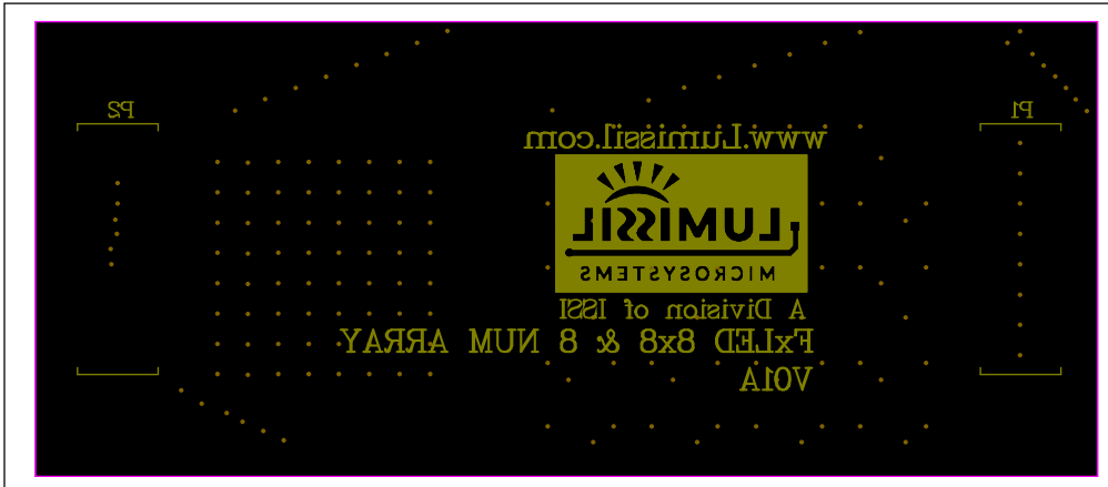
Figure 11: LED Board Component Placement Guide - Bottom Layer
