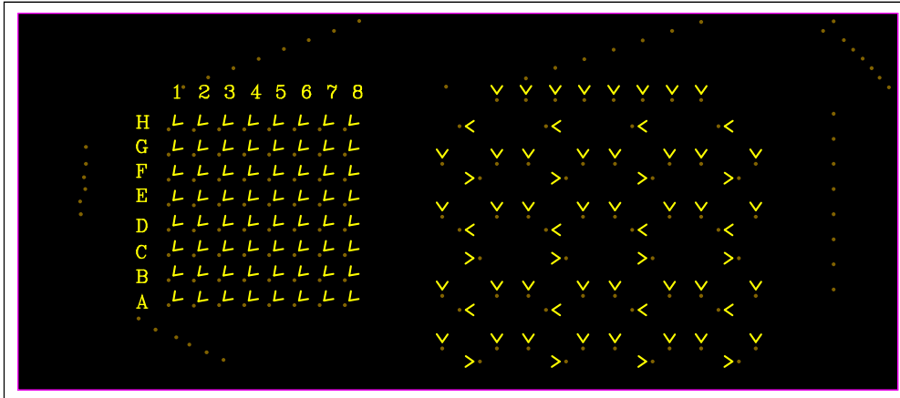
Figure 9: LED Board Component Placement Guide - Top Layer
