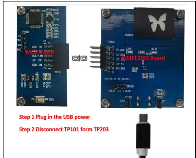
Figure 2: Photo of IS31FL3293 Board disconnected from MCU board
