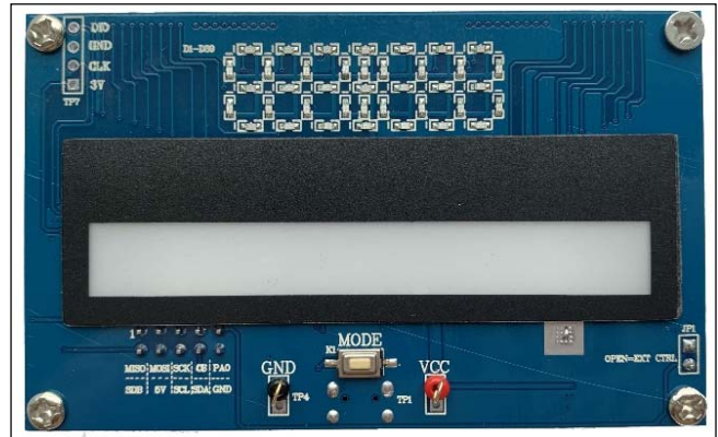
Figure 1: Photo of IS31FL3246A Evaluation Board
