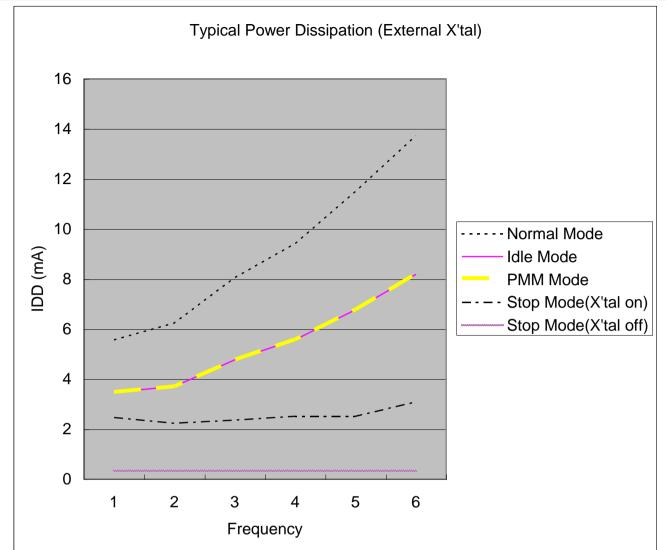
The values of performance frequency in IDLE and PMM modes are close therefore the lines appear overlapped in the graph.
