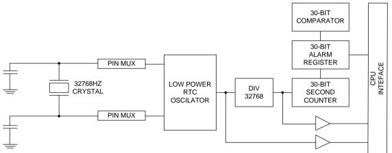
aThe RTC oscillator is enabled by RTCEN bit in XOSCCFG register. When enabled, RTC oscillator consumes about 2.5uA. Please note RTCEN bit is only cleared by power-on reset and not by other types of reset. The software must set RTCEN to 1 to use the RTC. The RTCXIN and RTCXOUT crystal pins are multiplexed with GPIO port P1.4 and
