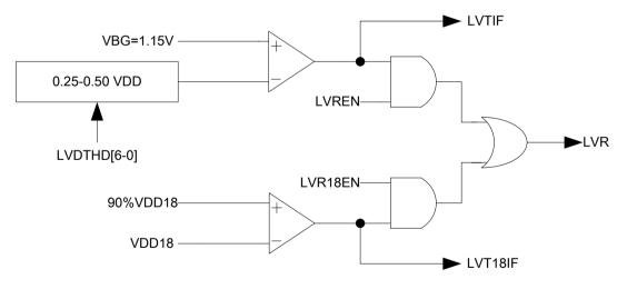
An enabled LVD circuit consumes about 100uA to 400uA depending on its VDD level. The LVDTHD[6-0] sets the compare threshold from 0.25VDD to 0.50VDD against the internal band-gap reference voltage of 1.15V. The detection threshold can be represented in the following equation when LVDTHV is the detection voltage.
