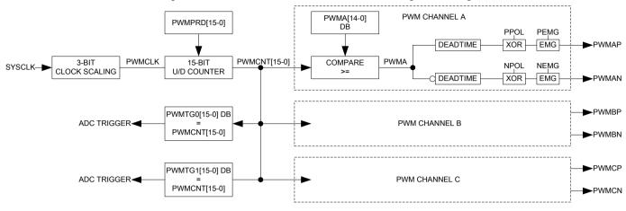
The period of the PWM frequency is defined by PWNPRD[14-0]. PWMPRD[15] is the enable control of the PWM and when read it represents up/down direction. A 15-bit Up/Down counter is used to provide the time base of the PWM channels. The operation of the PWM waveform is illustrated in the following timing diagram.
