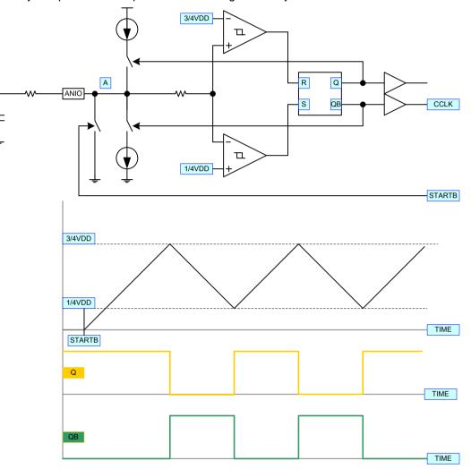
The touch detection algorithm is done in software and is assisted with the following hardware. The hardware consists of one 24-bit Timer and a 24-bit Counter. The clock into the timer and the counter can be interchanged by MODE selection.
