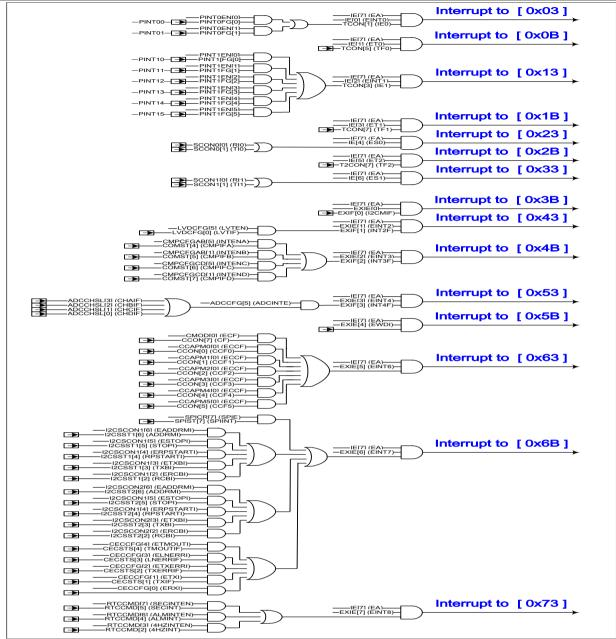
The interrupt related registers are listed in the following. Each interrupt can be individually enabled or disabled by setting or clearing corresponding bits in IE, EXIE and integrated peripherals' control registers.
