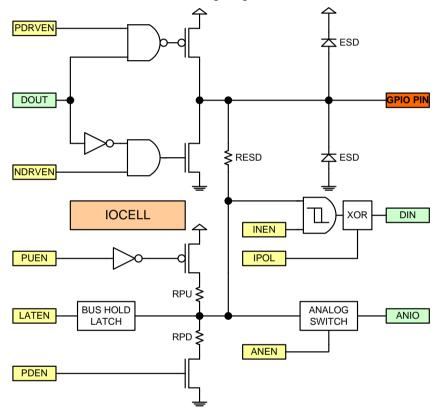
There are some variations of the IOCELL. IOCELLHP, IOCELLHN are IOCELL with high P drive and high N drive capabilities respectively. IOCELLHP can source up to 16mA, and IOCELLHN can sink up to 16mA. The configuration control of IOCELLHP and IOCELLHN is the same as IOCELL. IOCELL2A is IOCELL with two analog multiplexer switches, ANIO and ANIO1. The control of IOCELL2A uses IOCFG's ANEN1 to replace LATEN.
