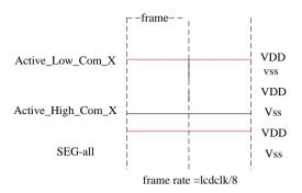
LCD 1/8 duty : display normal operation
