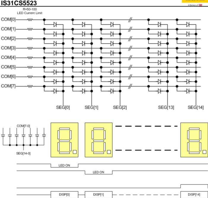
Since each SEG output needs to sink up to 8 LED if all COM output is enabled, the total sink current must be less than 8 x of COM source current. For sink current up to 125mA, the LED current thus should be limited to 125mA/8 = 16mA. Then the average LED current can be derived as  $16mA \times Duty$  Cycle. For example, total 10 digits are enabled then the average LED current is 1.6mA.
