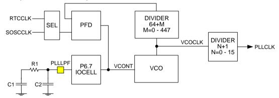
The PLL can be enabled or disabled. When enabled, it consumes approximately 500uA. The stabilization time of PLL requires about 10msec (M=256), and the stabilization time increases with M increases. Software should allow more than 20msec for PLL stabilization.
