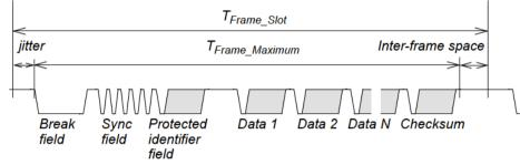
LIN bus protocol is based on frame. Each frame is partitioned into several parts as shown above. For master to initiate a frame, the software follows the following procedure.
