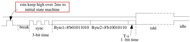
The sequence is initiated for RSTN=0 > 4msec (BREAK field), then followed by three SYNC bit, and two bytes sequence and a T-S bit. RSTN then must returned to 0 to maintain the test mode. If the sequence is not exactly matched, a BREAK field must be inserted to start over the sequence. The hardware block diagram is shown in the following and key parameters are also illustrated.
