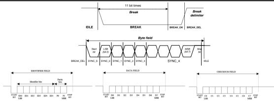
A LIN frame structure is shown and the frame time matches the number of bits sent and has a fixed timing.
