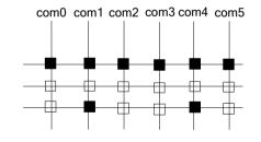
Reg\_Seg={com7,com6,com5,com4,com3,com2,com1,c om0} DISPDAT0=6'b111111 DISPDAT1=6'b000000 DISPDAT2=6'b010010
