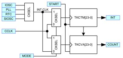
When MODE=0 (MODE0), the counter uses internal clock and timer uses sensing clock. This typically is used when the capacitance oscillation is slower. When MODE=1 (MODE1), the clock relationship is reversed and this is typically used when sensing oscillation is faster. Typical waveforms are shown in the following timing diagram.
