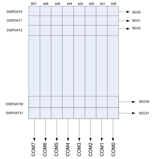
DISPDAT00~31 provide SEG00~31 output contents, output sequence follows COMx timing,
