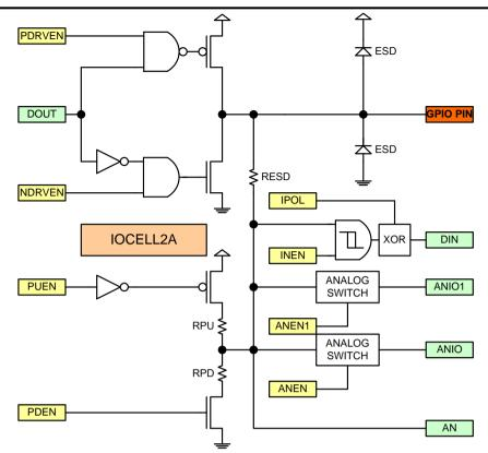
From the diagram, there are 7 control bits for the IOCFGPx.y register, and these registers are located at XFR 0xA040 – 0xA047 for P0.0 to P0.7, 0xA048 – 0xA04F for P1.0 to P1.7, 0xA060 – 0xA067 for P2.0 to P2.7, and 0xA068 – 0xA06F for P3.0 to P3.7. The definitions of IOCFGPx.y are described in the following table.
