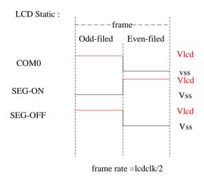
frame rate =30Hz sysclk = 16Mhz, T2M=0 , div-12 timer2-value = 16\*2^20 /12/30/2 = 23302 {TP2H,TP2L}=2^16-23302 = 16'hA4FA
