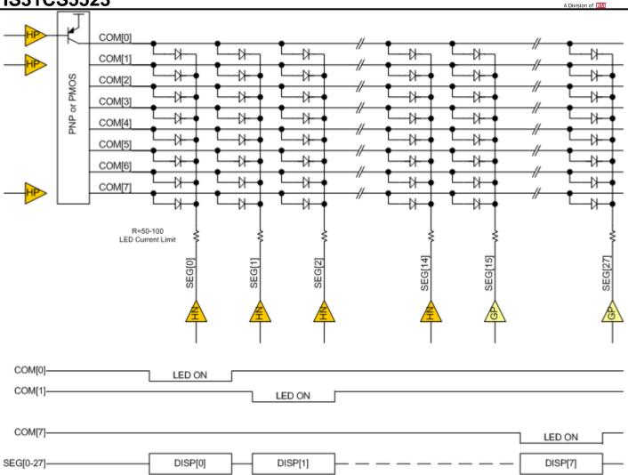
In the example, COM output is connected to external PNP or PMOS transistor to supply LED current. In this case, COM output polarity must be set in order to obtain correct driving signals. When PNP is used, maximum LED brightness should be set to 63/64 in order to avoid ghosting due to PNP extended turn-off delay. Alternatively, NPN transistors can also be used. NPN transistor can also serve as high voltage blocking function for LED array.
