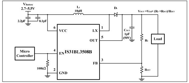
Figure 4 Constant Output Voltage For General Purpose Use
