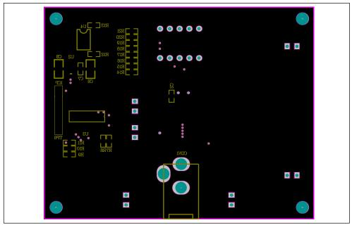
Figure 5: Board Component Placement Guide -Bottom Layer
