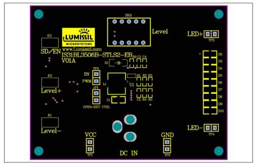
Figure 3: Board Component Placement Guide -Top Layer
