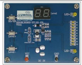
Figure 1: Photo of IS31BL3506B Evaluation Board
