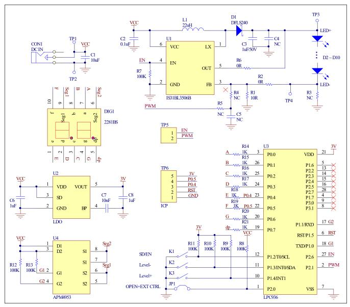
Figure 2: IS31BL3506B Application Schematic
