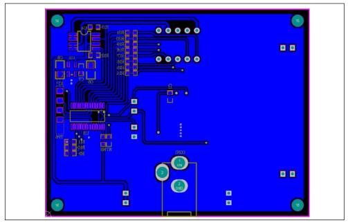
Figure 6: Board PCB Layout-Bottom Layer
