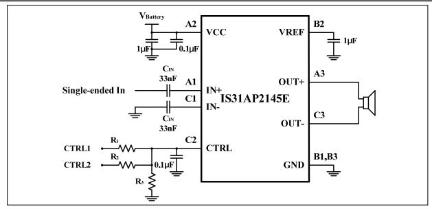
Figure 2 Typical Application Circuit (Single-Ended Input)
