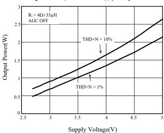
Figure 11 Output Power vs. Supply Voltage
