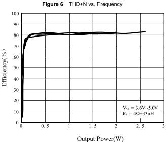
Figure 8 Efficiency vs. Output Power
