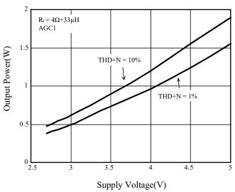
Figure 12 Output Power vs. Supply Voltage
