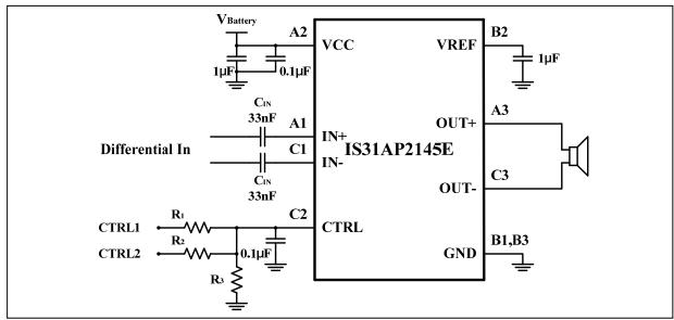
Figure 1 Typical Application Circuit (Differential Input)
