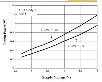
Figure 10 Output Power vs. Supply Voltage
