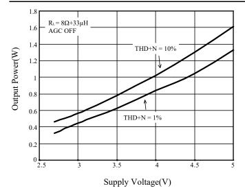
Figure 9 Output Power vs. Supply Voltage
