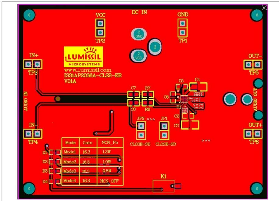
Figure 4: Board PCB Layout - Top Layer
