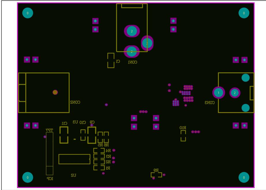
**Figure 5: Board Component Placement Guide - Bottom Layer**
