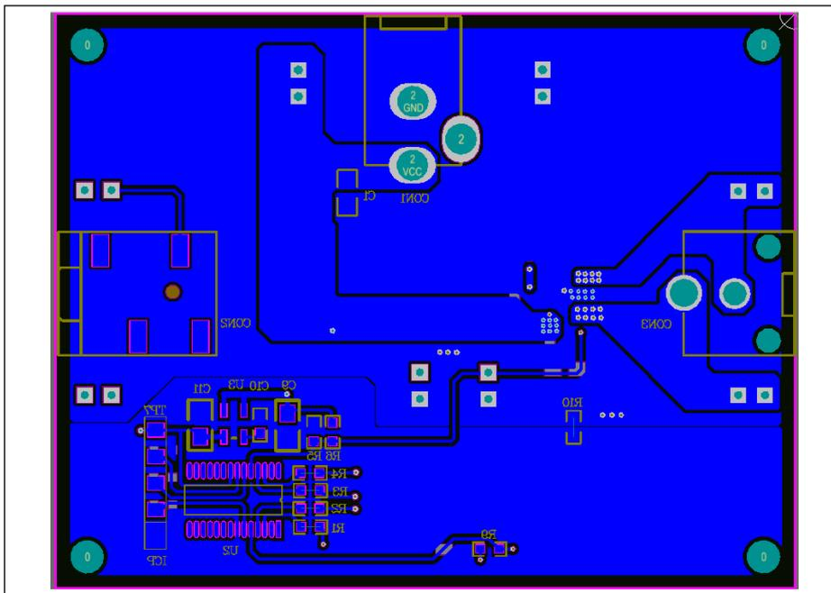
**Figure 6: Board PCB Layout - Bottom Layer**
