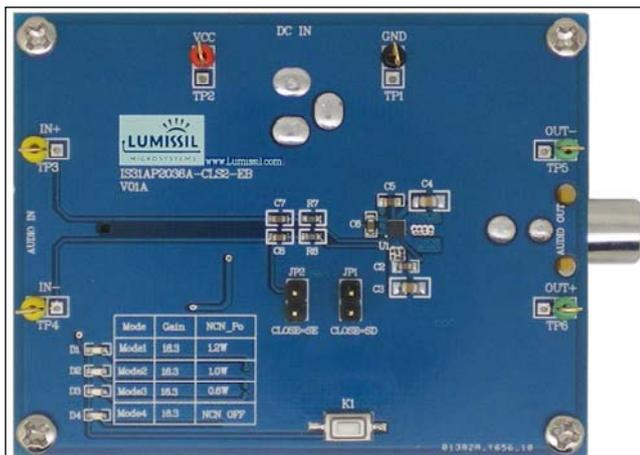
Figure 1: Photo of IS31AP2036A Evaluation Board
