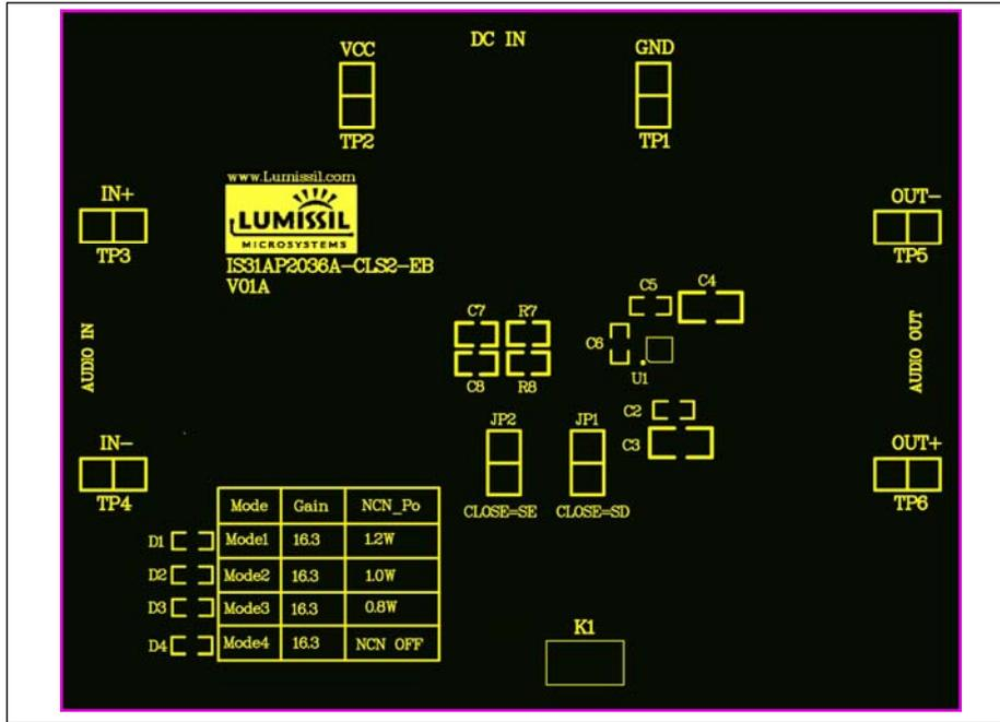
Figure 3: Board Component Placement Guide - Top Layer
