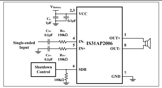
Figure 2 Typical Application Schematic (Single-ended Input)
