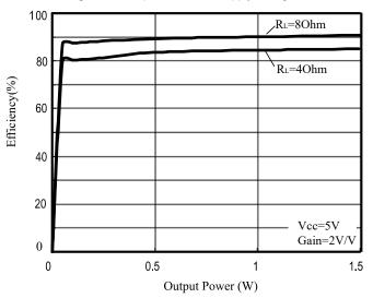
Figure 11 Efficiency vs. Output Power
