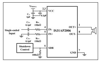
Figure 13 Typical Application Circuit with Single-Ended Input
