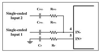
Figure 16 Application Circuit with Summing Two Single-Ended Inputs
