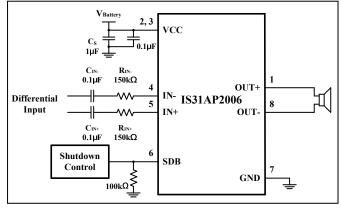
Figure 12 Typical Application Circuit with Differential Input
