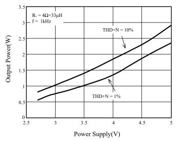
Figure 10 Output Power vs. Supply Voltage
