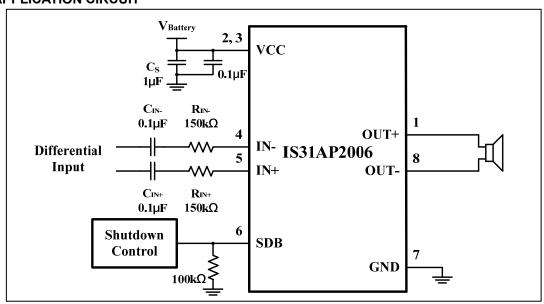
Figure 1 Typical Application Circuit (Differential Input)
