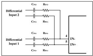
Figure 14 Application Circuit with Summing Two Differential Inputs
