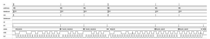
Figure-45. Receiving 3 Bytes Followed By Repeated Start And Sending 3 Bytes Waveform
