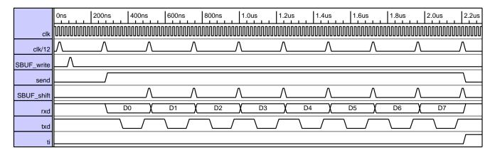
Figure-18. UARTO Transmission Mode 0 Timing Diagram
