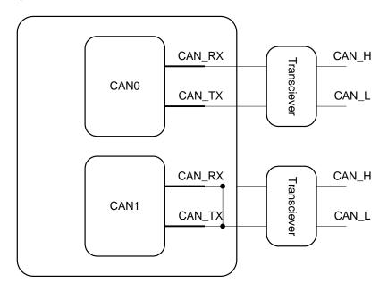
Figure-83. CAN1 In Self-loop Test
