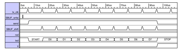
Figure-19. UARTO Transmission Mode 1 Timing Diagram
