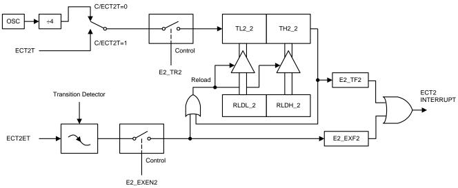
Figure-62. ECT2 Auto-Reloaded Mode
