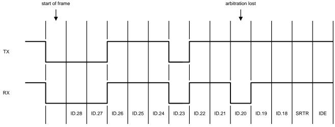
Figure-74. Example 0f arbitration Lost Bit number Interpretation; Result: ALC = 08H
