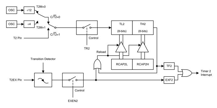
Figure-15. Timer 2 Auto-reloaded Mode (DCEN =0)
