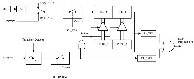
Figure-60. ECT1 Auto-Reloaded Mode
