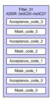
Figure-77. CANO Acceptance Filters
