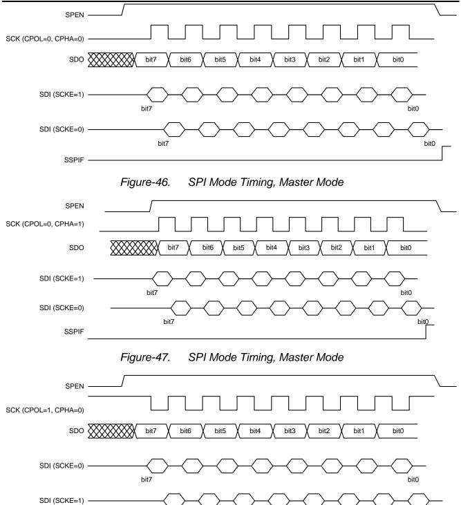
Figure-48. SPI Mode Timing, Master Mode
