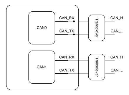
Figure-82. CANO In Self-Loop Test
