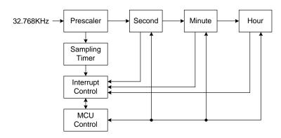
Figure-55. RTC Configuration
