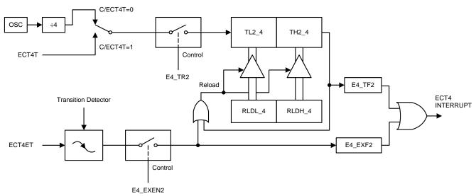
Figure-66. ECT4 Auto-Reloaded Mode
