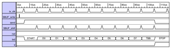
Figure-25. UART1 Transmission Mode 3 Timing Diagram
