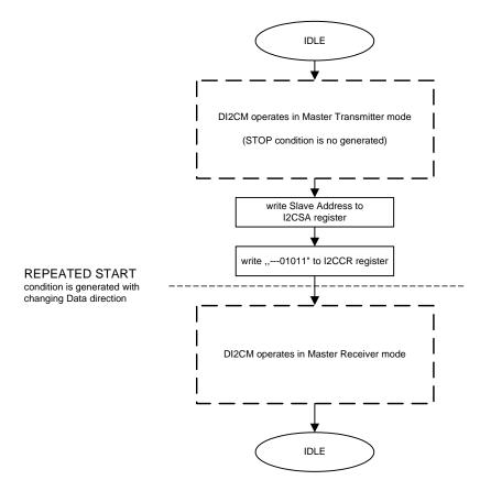
Figure-42. Sending n Bytes Followed By Repeated Start And Receiving m Bytes Flowchart
