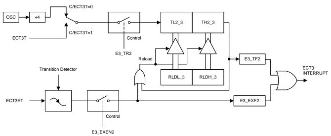
Figure-64. ECT3 Auto-Reloaded Mode
