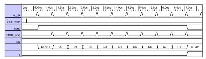
Figure-20. UARTO Transmission Mode 2 Timing Diagram
