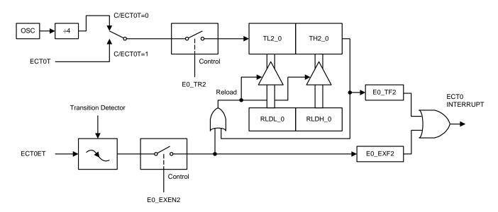
Figure-58. ECT0 Auto-Reloaded Mode
