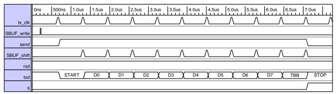
Figure-24. UART1 Transmission Mode 2 Timing Diagram
