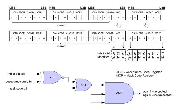
Figure-80. Filter 0 in CAN0 Is Receiving Standard Frame Messages
