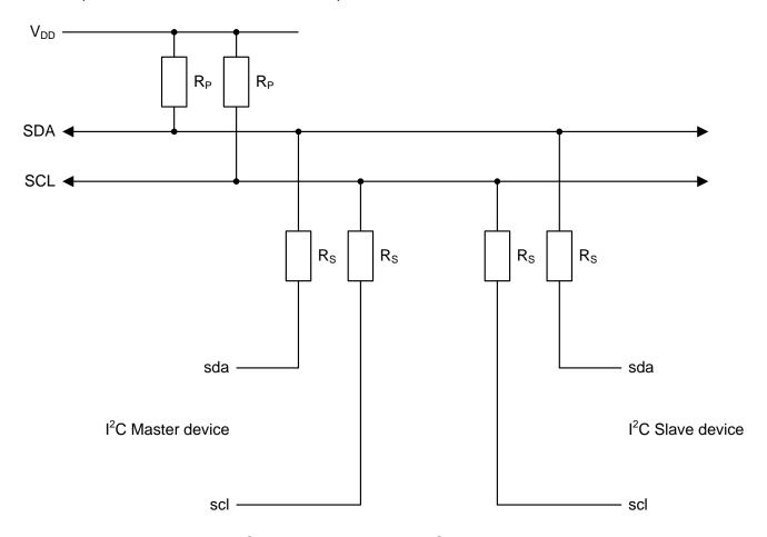
Figure-27. Connection Master And Slave Devices To I2c-Bus
