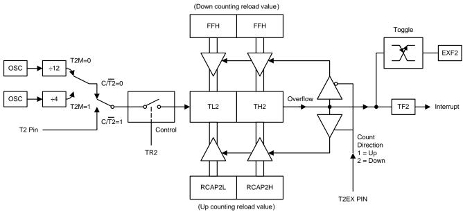
Figure-16. Timer 2 Auto-Reloaded Mode (DCEN =1)
