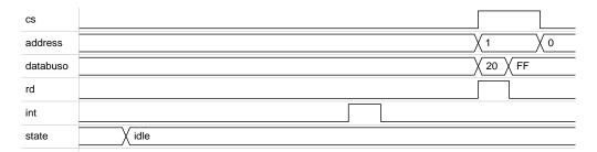
Figure-35. Single SEND Waveform - STATUS REGISTER READING
