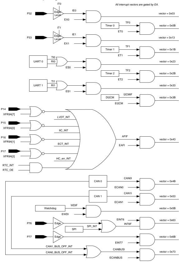
Figure-5. Interrupt Diagram
