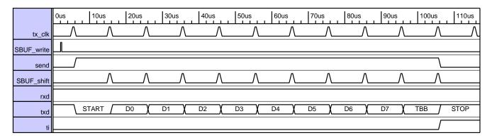
Figure-21. UARTO Transmission Mode 2 Timing Diagram
