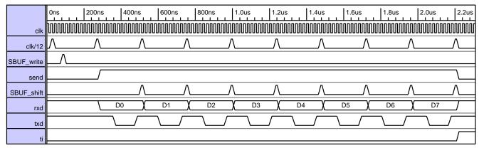
Figure-22. UART1 Transmission Mode 0 Timing Diagram
