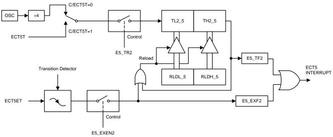
Figure-68. ECT5 Auto-Reloaded Mode
