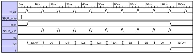
Figure-23. UART1 Transmission Mode 1 Timing Diagram
