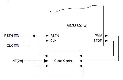
Figure-6. Power Saving Unit Interconnection
