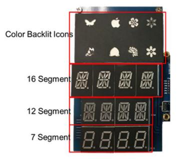
All three drivers are controlled via 1MHz I2C interface; permitting highspeed register write or read. The IS31FL3716 can control each individual LED on/off with 128 steps of global current control for white balance adjustment. This means each LED will have 1 brightness level but adjusted for pure white color.
